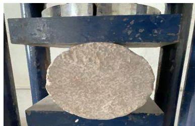
Figure 3. Tensile Strength on Cylindrical Specimen
