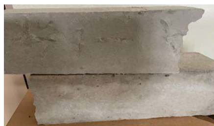
Figure 4. Failed Beam Specimen from UTM
