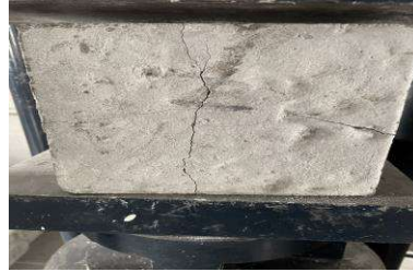
Figure 2. Compressive Strength test cubic Specimen FAA Concrete
