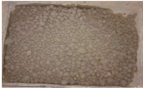
Figure 1. Sintered Fly Ash Aggregates
