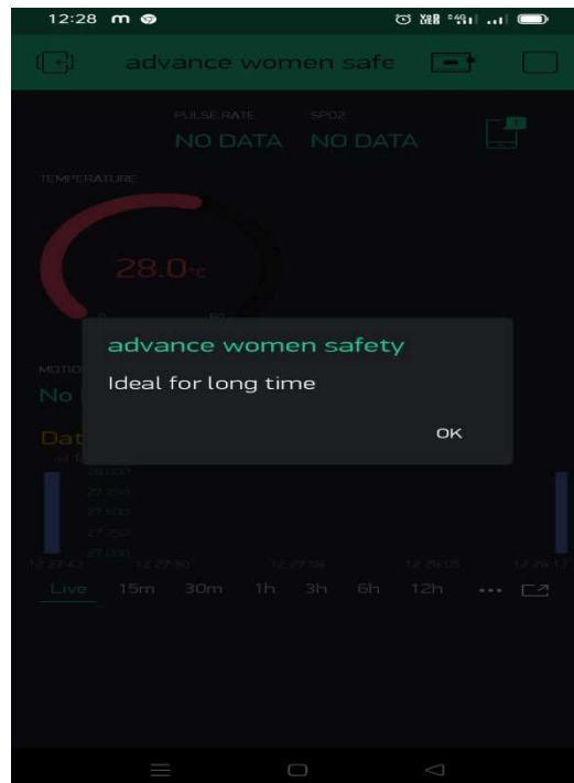
Fig 8: Alert message if no motion is detected for the set threshold value
