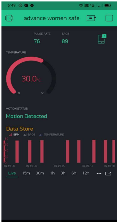
Fig 6: Values of pulse rate, spo2, temperature, motion status and data store chart in blynk app.
