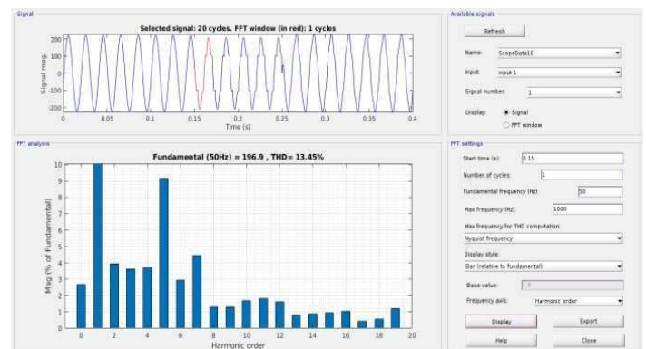
Fig 8.Total harmonic distortion of the compensated voltage
