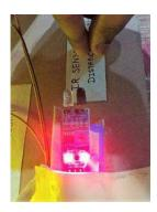
If there is not enough distance between two individuals, then the LED on the IR Sensor will be lit and the buzzer will also start ringing.
